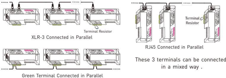
5.3 The connection diagram of AMP signal amplifier terminal:
