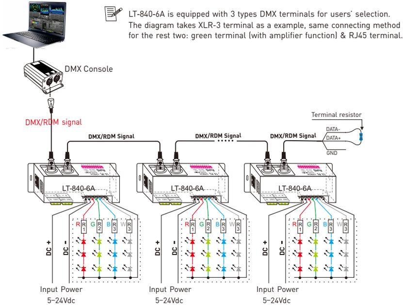
LT-840-6A is equipped with 3 types DMX terminals for users' selection. The diagram takes XLR-3 terminal as an example, same connecting method for the rest two: green terminal (with amplifier function) & RJ45 terminal.
